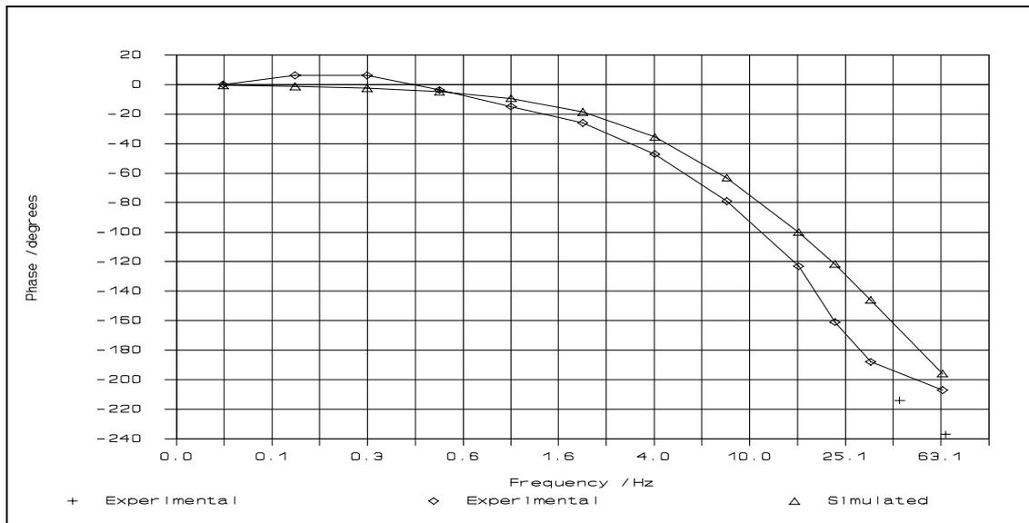
**Figure 5.9** Bode plot (phase) for the position response of the heave mode suspension
