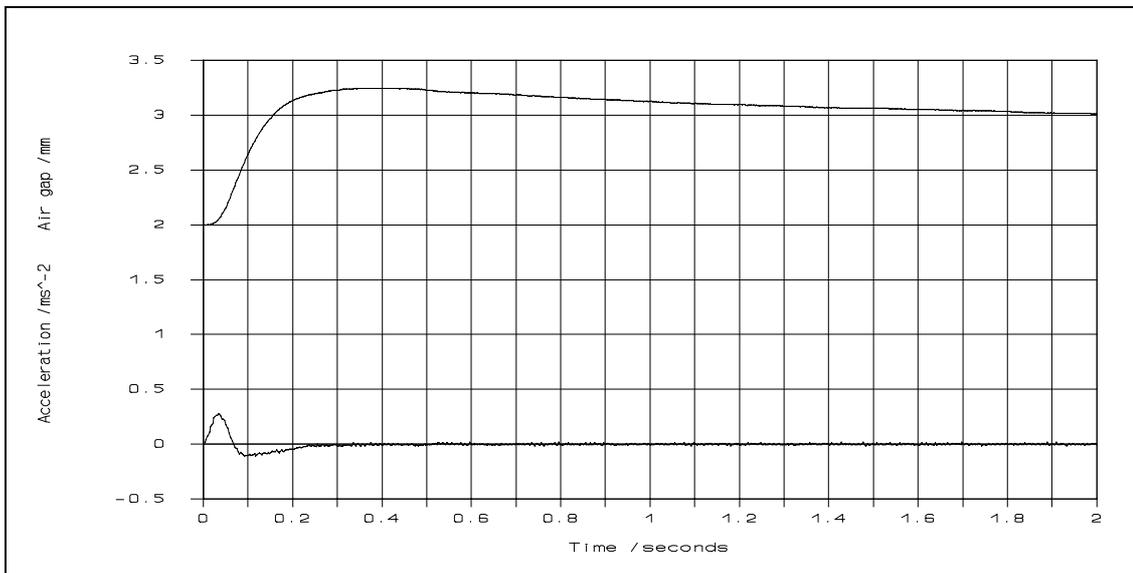
**Figure 5.14** Experimental heave response to a 1 mm simulated track step (80 kg passenger)
