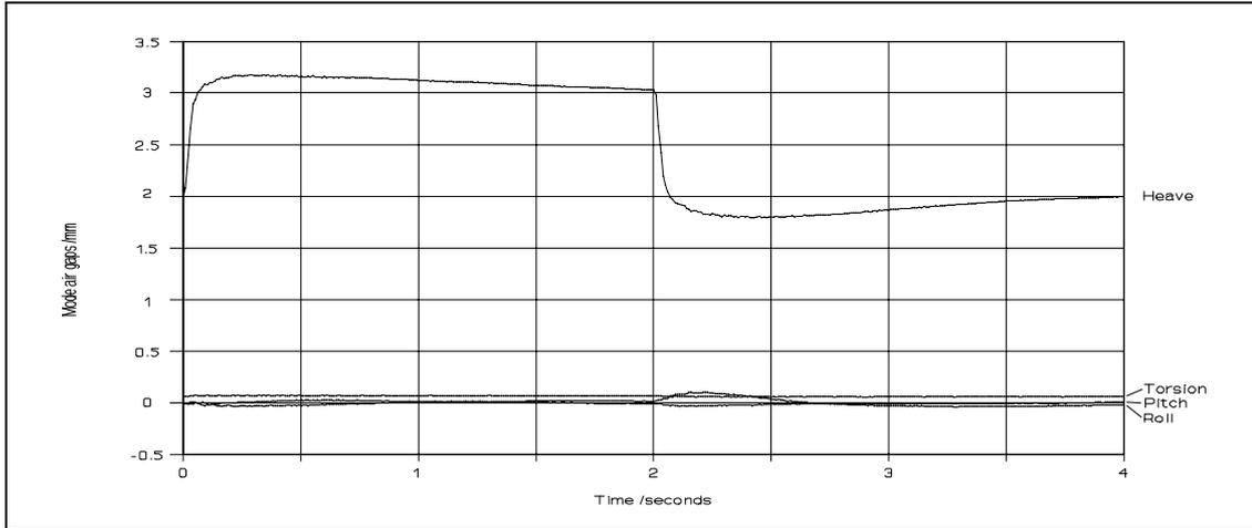
Figure 5.10 Experimental mode responses to a 1 mm *heave* position reference step
