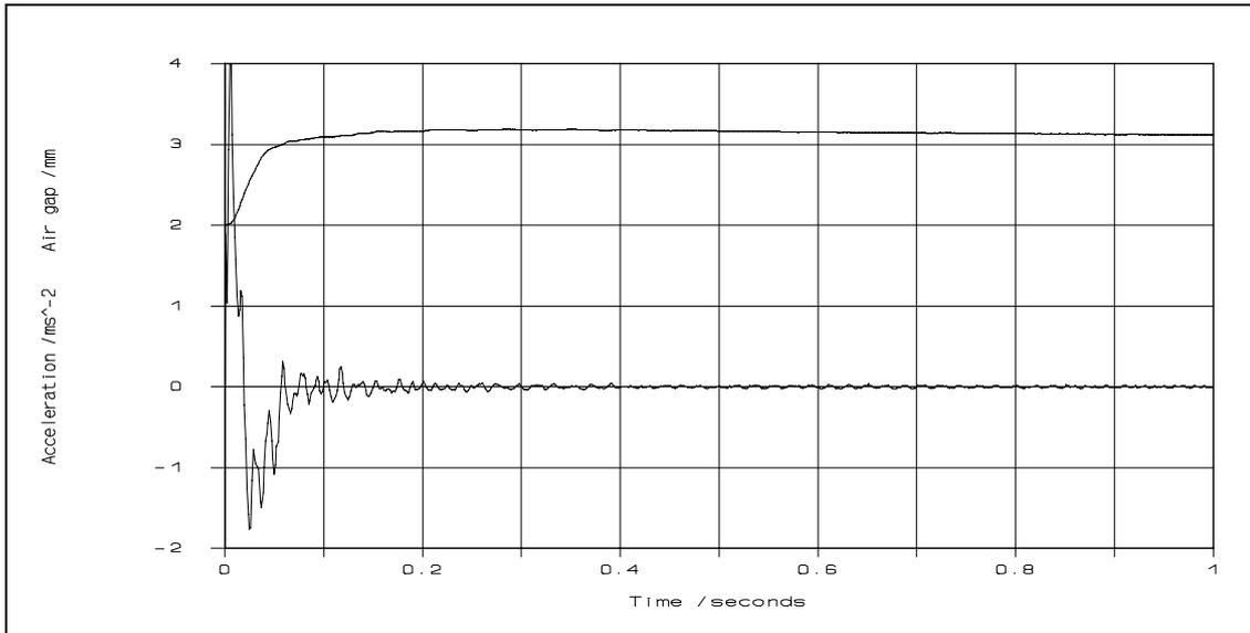
**Figure 5.4** Experimental heave response to a 1 mm position reference step (no passenger)
