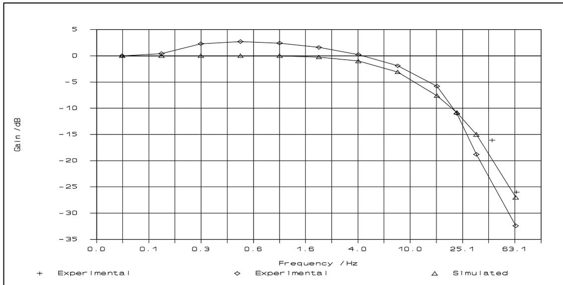
**Figure 5.8** Bode plot (gain) for the position response of the heave mode suspension
