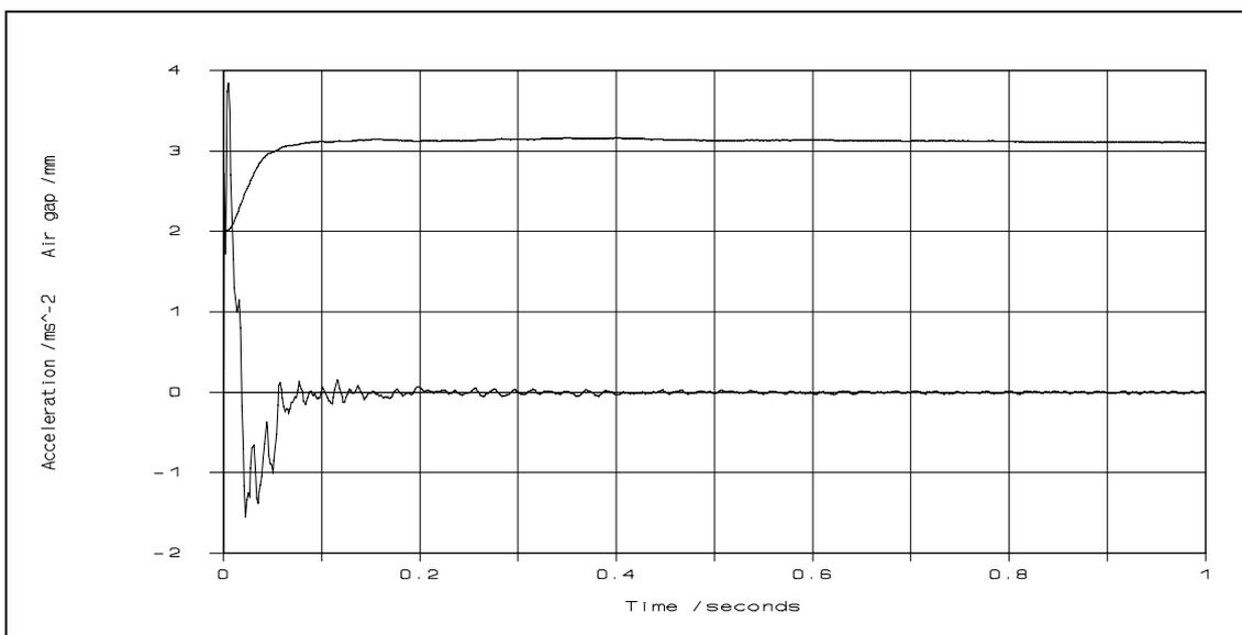
**Figure 5.5** Experimental heave response to a 1 mm position reference step (80 kg passenger)
