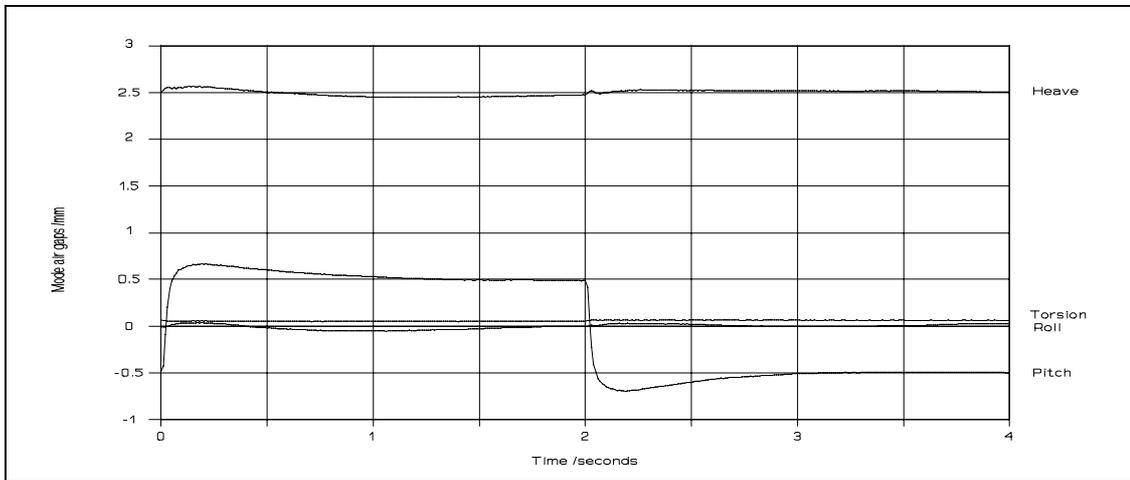
Figure 5.11 Experimental mode responses to a 1 mm *pitch* position reference step
