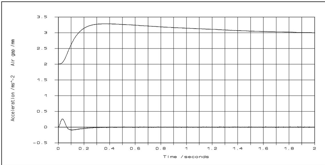
**Figure 5.13** Experimental heave response to a 1 mm simulated track step (no passenger)
