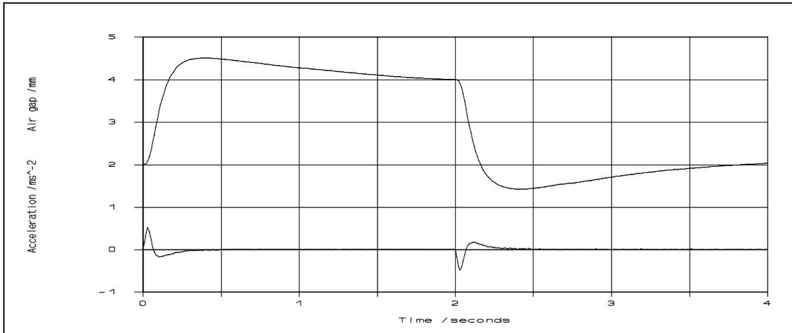
Figure 5.15 Experimental heave response to a 2 mm simulated track *heave* step
