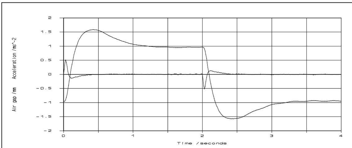
Figure 5.17 Experimental roll response to a 2 mm simulated track *roll* step
