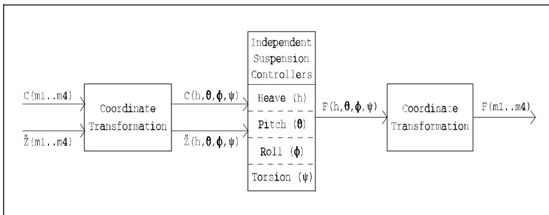
Figure 5.3 Configuration of the vehicle suspension control system
