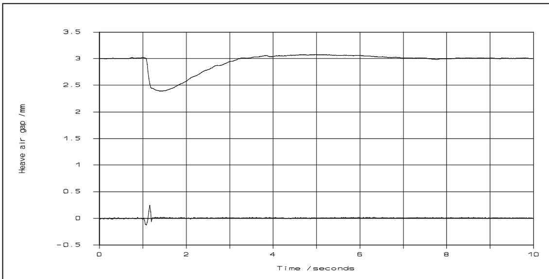
**Figure 5.6** Experimental heave response to a 500 N heave disturbance force
