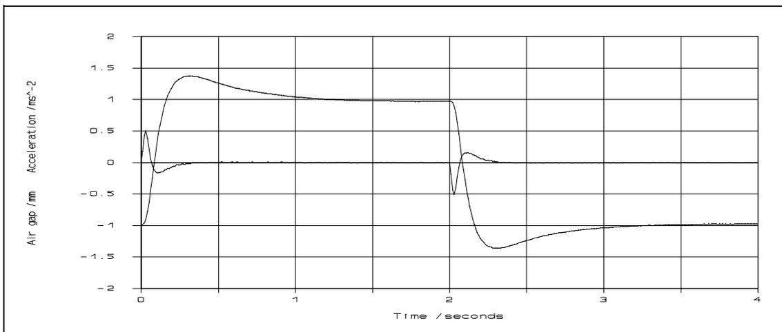
Figure 5.16 Experimental pitch response to a 2 mm simulated track *pitch* step
