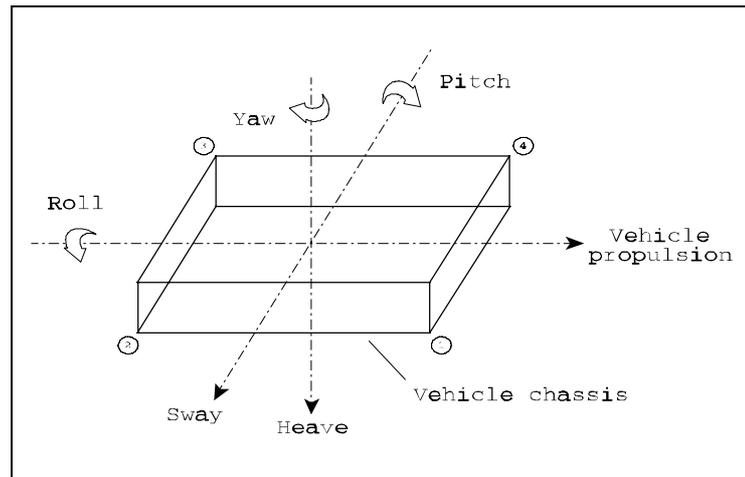
**Figure 5.2** Free-body motion of the vehicle
