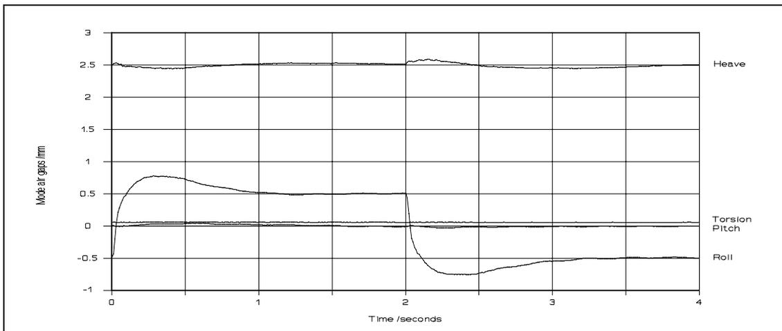
Figure 5.12 Experimental mode responses to a 1 mm *roll* position reference step
