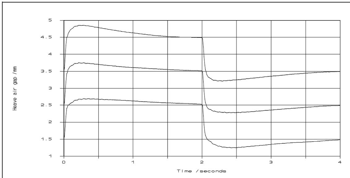
**Figure 5.7** Experimental heave responses to three 1 mm heave position reference steps
