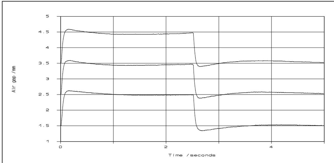
**Figure 4.10** Experimental suspension responses to three 1 mm air gap reference steps ( $\omega_{follow} = \infty$  rad/s,  $m = 30$  kg)
