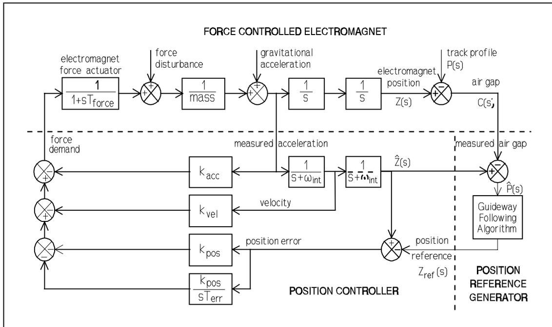
Figure 4.4 Suspension control system configuration
