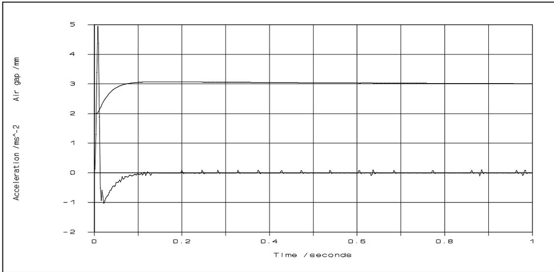
**Figure 4.6** Simulated suspension response to a 1 mm air gap reference step
