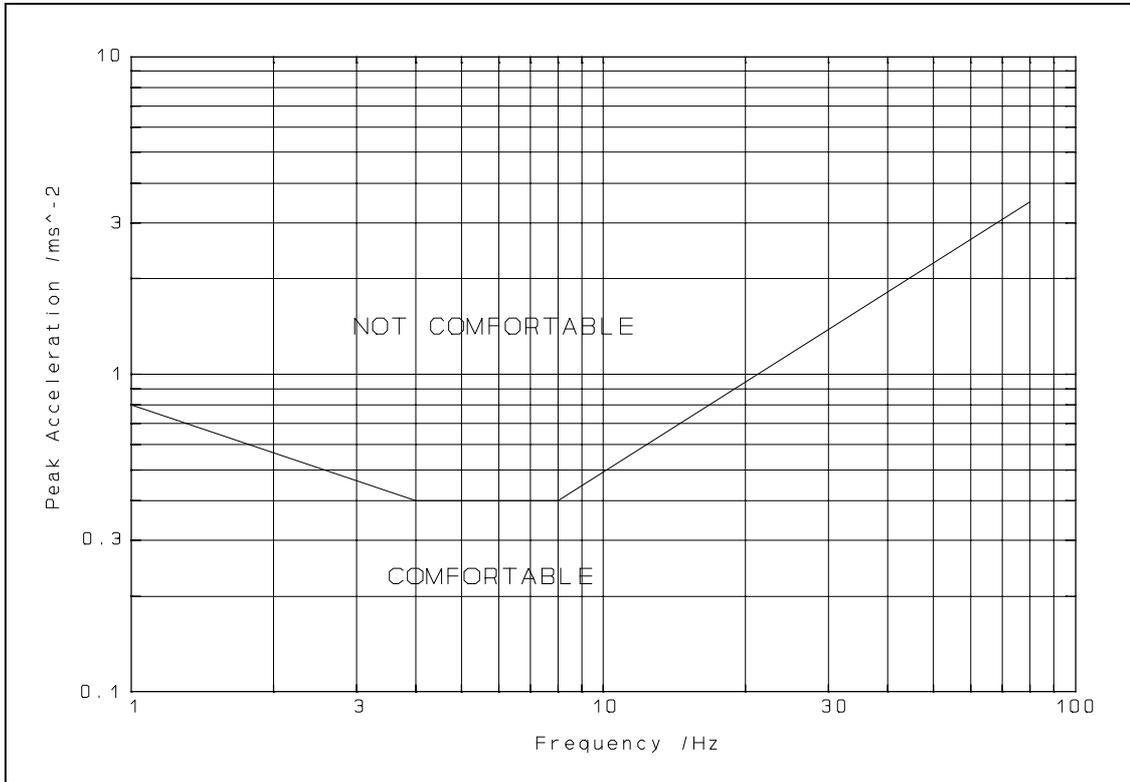
**Figure 4.1** ISO reduced comfort boundary (for a 1 hour exposure)
