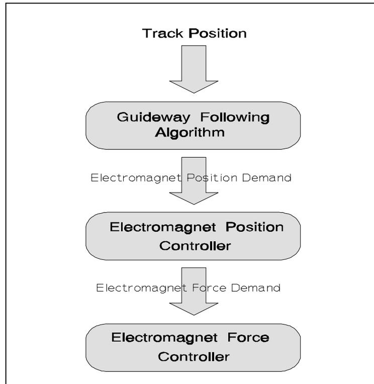
**Figure 4.2** Suspension control system hierarchy
