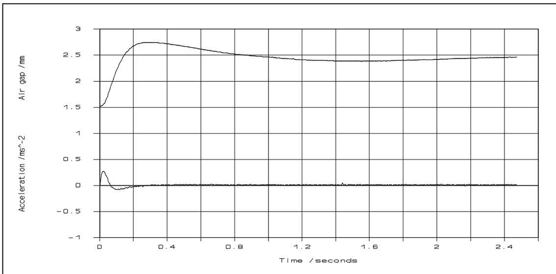
**Figure 4.12** Experimental suspension response to a 1 mm simulated track step ( $m = 15$  kg)
