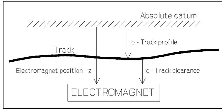
Figure 4.3 Logical arrangement of the suspension system
