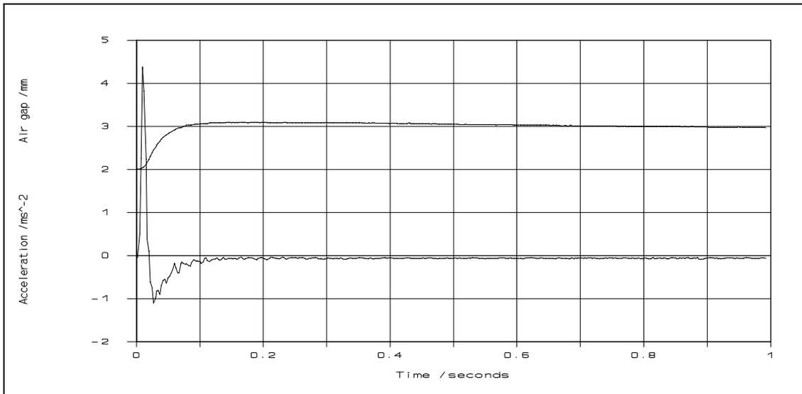
**Figure 4.7** Experimental suspension response to a 1 mm air gap reference step
