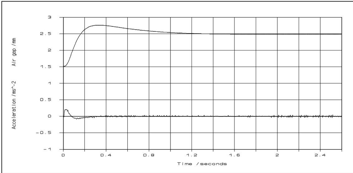
**Figure 4.11** Simulated suspension response to a 1 mm simulated track step ( $m = 15$  kg)
