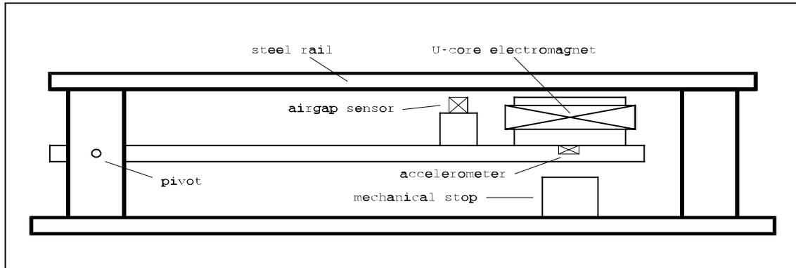
**Figure 4.5** Single electromagnet suspension experimental rig
