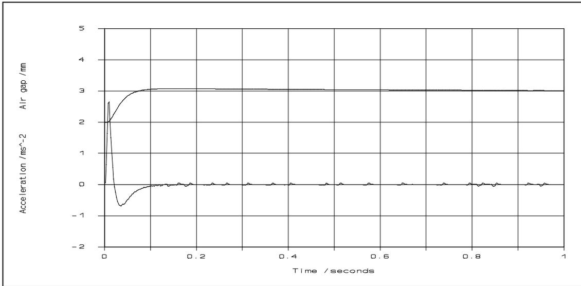
**Figure 4.8** Simulated suspension response to a 1 mm air gap reference step
