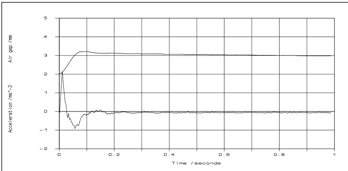
**Figure 4.9** Experimental suspension response to a 1 mm air gap reference step
