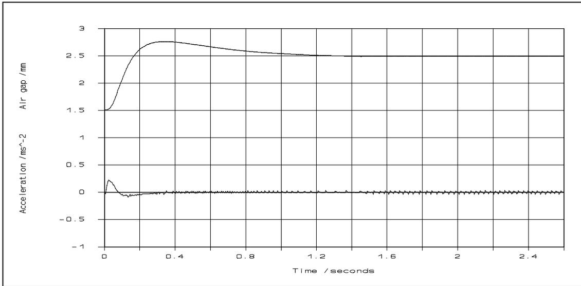
**Figure 4.13** Simulated suspension response to a 1 mm simulated track step ( $m = 45$  kg)
