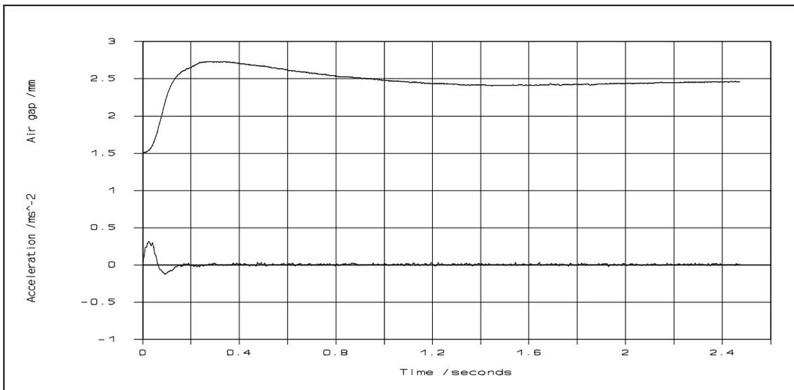
**Figure 4.14** Experimental suspension response to a 1 mm simulated track step ( $m = 45$  kg)
