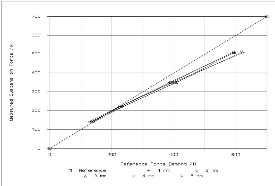
**Figure 3.8** Experimental controller reference force demands and actual suspension forces
