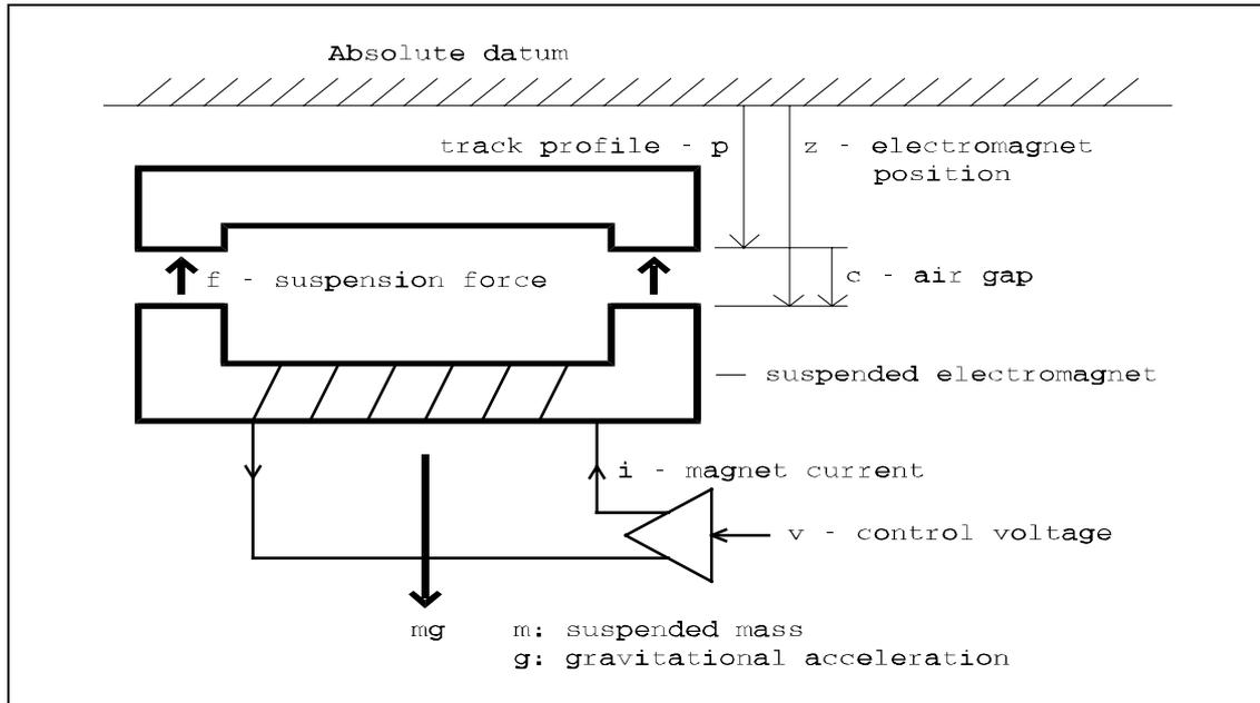
**Figure 3.1** Electromagnet and track configuration
