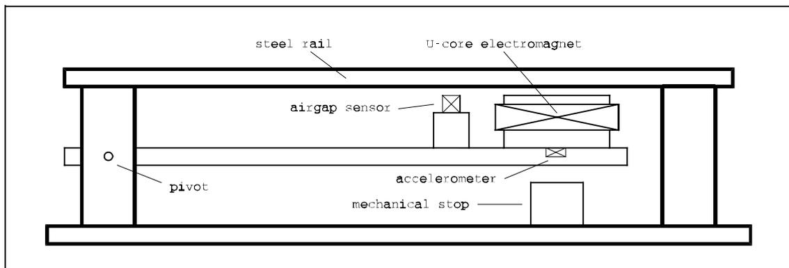
**Figure 3.7** Single electromagnet suspension experimental rig
