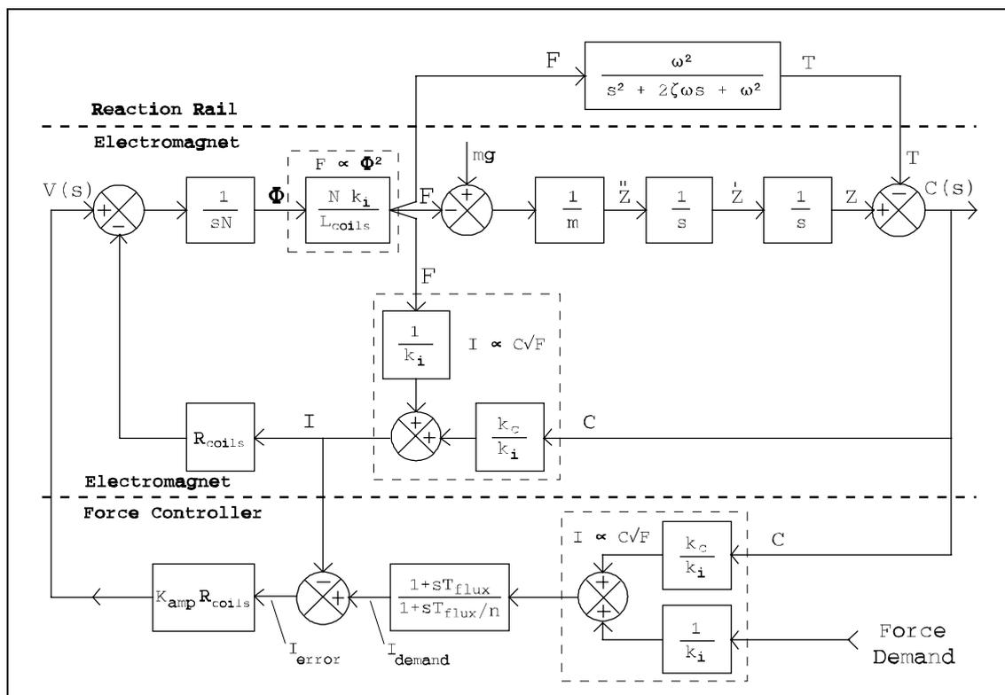
Figure 3.5 Proposed force control configuration
