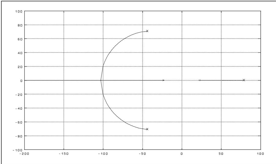
**Figure 3.3** Closed-loop root locus for force feedback
