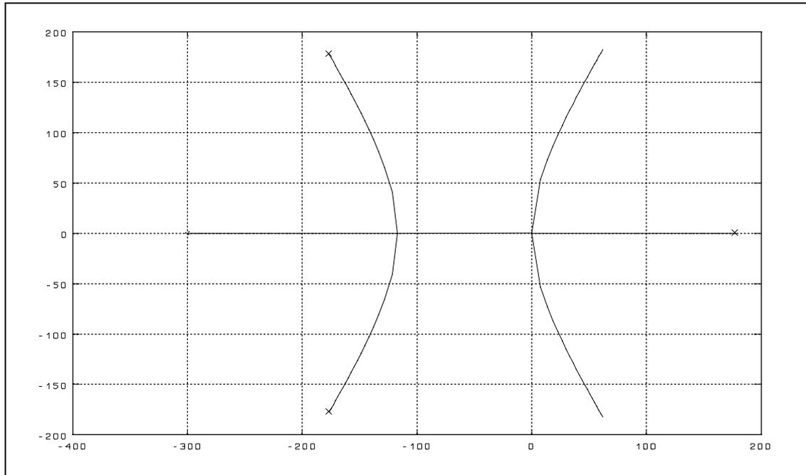
**Figure 3.4** Closed-loop root locus for air gap and current feedback
