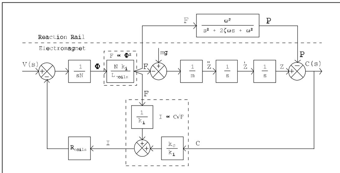
Figure 3.2 Block diagram of the electromagnet system
